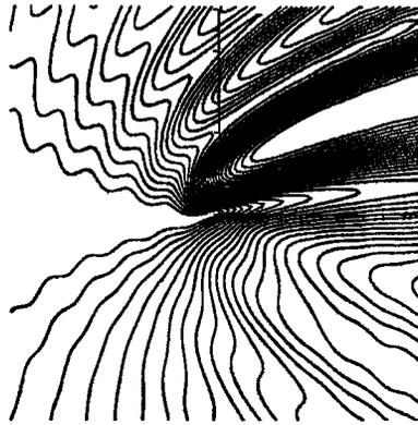
FIGURE 4. Iso-contours of the root-mean-square pressure level of the scattered wave, normalized by the amplitude of incident wave. Contour levels: Minimum = 0.08; Maximum = 1.12; Increment = 0.04. ( $\epsilon = 0.27$ ,  $\lambda/L = 4$ ,  $M = 0.125$ ).
